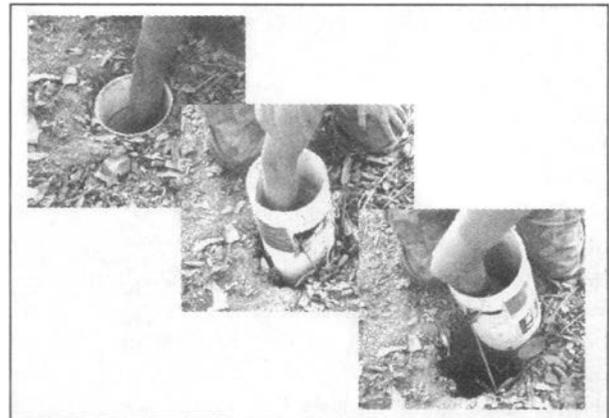
Fig. 5. The passive trigger closes the snare's loop when the PVC pipe is pulled out of the ground by hooking the screen fixed within the bottom of the pipe.
