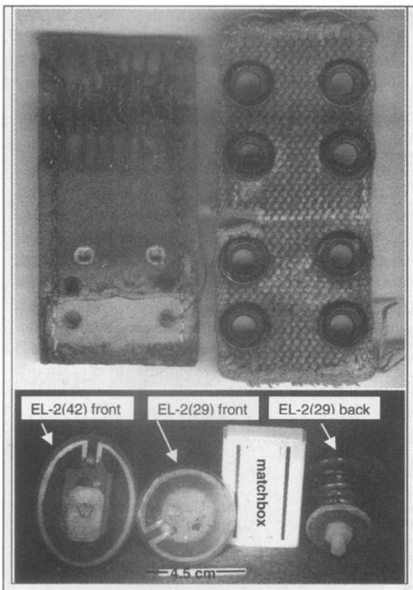
**Fig. 2.** Breakaway devices used on radiotrigger collars in Slovenia, 1993–98. Top: Collar featured either 18 loops of 1-mm iron wire (left) or cotton spacers (cotton webbing links with grommets, right). For subadult bears, collars were notched on one or both edges to allow for a more rapid break off. Bottom: Eartag transmitters (used after 1996) weighed 42 g (EL-2[42]) and 29 g (EL-2[29])g.
