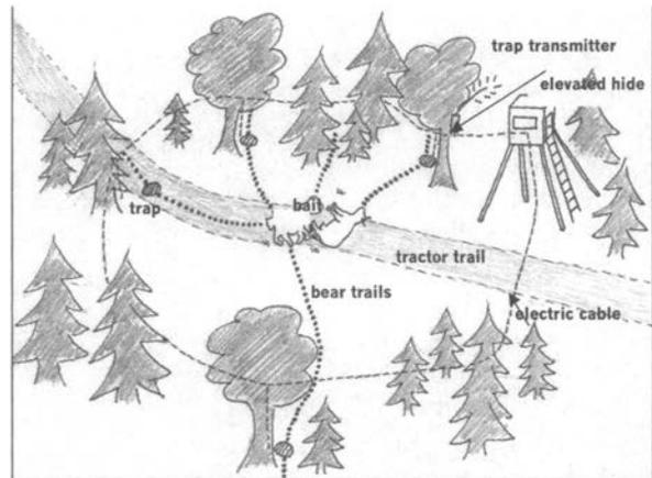
Fig. 1. Schematic of trap site and alarm system used to capture bears in Slovenia, 1993–98. Two to 6 traps were arranged at each bait site, connected with each other and a trap transmitter. The trap transmitter was mounted in a tree to allow for a reception range up to 30 km. Electric wires connecting the traps and transmitter were mounted 2–3 m above ground to avoid problems with rodents.
